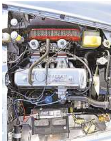
This 1,982cc four-cylinder engine, left, is original to the car, Mr. Davidson says. Detail of the car's interior, right. The original upholstery is vinyl. He bought the car in 2006.
